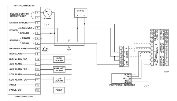
Figure 11—A Typical System, Infiniti Transmitter with PointWatch Wired to R8471 Controller, Non-Isolated Current Output
