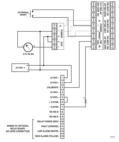
NOTES: 1 250 OHM RESISTOR REQUIRED IF USING HART PORT COMMUNICATIONS.
