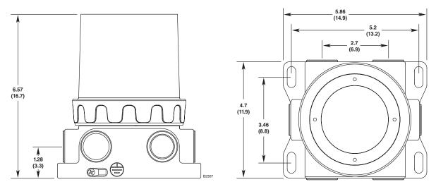
NOTE: TO MOUNT THE TRANSMITTER, DRILL 5/6" (7.9375mm) HOLES AND USE 1/4" (6.35mm) BOLTS.
