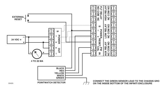
Figure 9—A Typical System - Infiniti Transmitter with a PointWatch Detector and Non-Isolated Current Output
