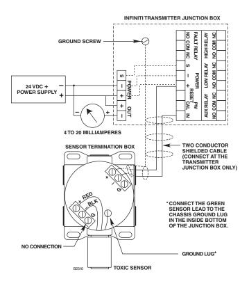
Figure 16—Sensor Separation with Toxic\* and Oxygen Gas Sensors and Infiniti Transmitter
