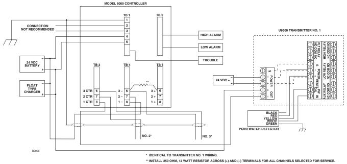
THIS RESISTOR WILL SATISFY POWER MONITORING REQUIREMENTS (ONLY CHANNEL 3 SHOWN FOR CLARITY).
