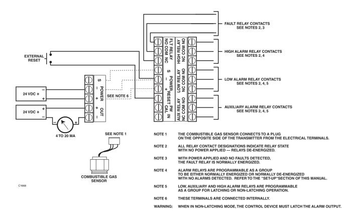
Figure 7—A Typical System - Infiniti Transmitter with Combustible Gas Sensor, Isolated Current Output and Relay Outputs
