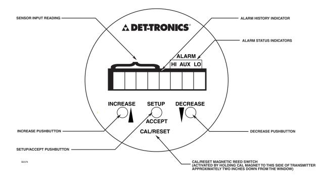
Figure 18—Infiniti Transmitter Controls and Indicators
