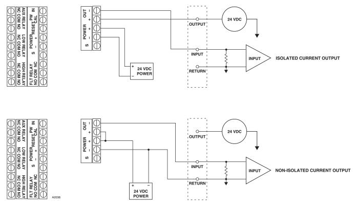
Figure 13—A Typical System, Infiniti Transmitter used with PLC Analog Input Module, Isolated/Non-Isolated Current Output
