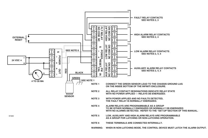
Figure 8—A Typical System - Infiniti Transmitter with a Toxic Gas / Oxygen Sensor, Non-Isolated Current Output and Relay Outputs
