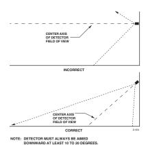
Figure 1—Detector Orientation Relative to Horizon
