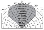
Field of View at Indicated Distance in Feet (m) for Methanol at Very High Sensitivity (1 x 1 foot)
