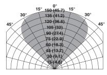
Field of View at Indicated Distance in Feet (m) for **Diesel** at **Very High** Sensitivity (1 x 1 foot)
