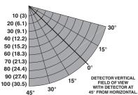
Field of View at Indicated Distance in Feet (m) for **Methane** at **Very High** Sensitivity (30 inch plume)
