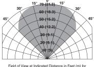
Field of View at Indicated Distance in Feet (m) for Methanol at Medium Sensitivity (1 x 1 foot)
