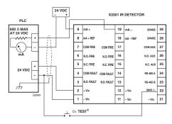
Figure 11—X3301 Detector Wired for Isolated 0 to 20 mA Current Output (Sourcing)
