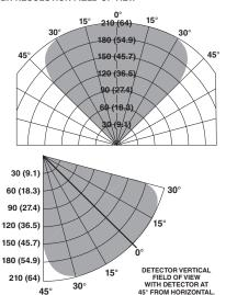
Field of View at Indicated Distance in Feet (m) for **n-Heptane** at **Very High** Sensitivity (1 x 1 foot)
