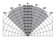
Field of View at Indicated Distance in Feet (m) for JP-5 at Medium Sensitivity (2 x 2 foot)
