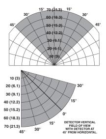
Field of View at Indicated Distance in Feet (m) for **Isopropanol** at **Very High** Sensitivity (6 in. x 6 in.)
