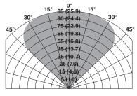
Field of View at Indicated Distance in Feet (m) for **Ethanol** at **Medium** Sensitivity (1 x 1 foot)
