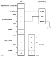
Figure 3-50—Electrochemical Sensor Connected to DCU
