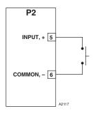
Figure 3-4—Unsupervised Input Wiring
