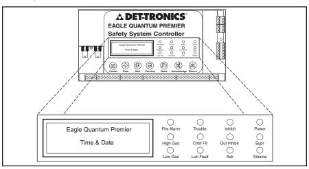
Figure 4-2—EQP Controller Message Display and System Status Indicator Location
