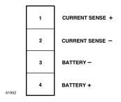
Figure 3-18—J2: Battery Test Points
