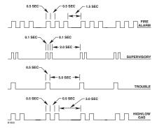
Figure 4-4—Tone Pattern for Controller Buzzer
