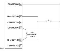
Figure 3-24—Supervised Input Configuration - Class A
