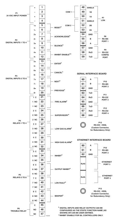
Figure 3-7—EQP Controller Terminal Identification
