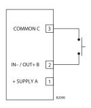
Figure 3-36—Unsupervised Input Configuration
