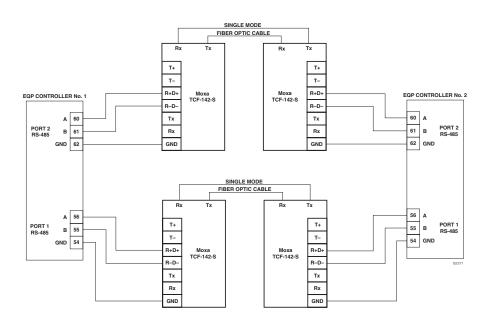
Figure 3-11—Single Mode Controller to Controller NFPA 72 Approved Fiber Optic Link, Class X
