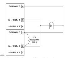
Figure 3-31—Supervised Output Configuration (Notification)— Class A
