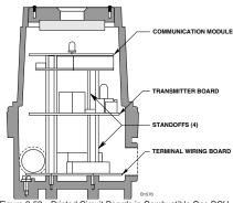
Figure 3-53—Printed Circuit Boards in Combustible Gas DCU
