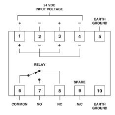
NOTE: RELAY CONTACTS ARE SHOWN IN THE REST STATE, NO POWER APPLIED. RELAY IS ENERGIZED WITH POWER APPLIED AND NO GROUND FAULT (TERMINALS 6 & 7 CLOSE, TERMINALS 6 & 8 OPEN).
