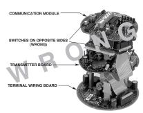
INCORRECT ORIENTATION OF TRANSMITTER BOARD
