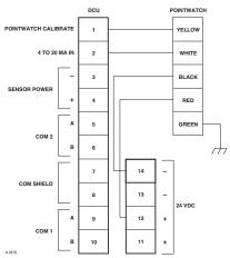
Figure 3-51—PointWatch/DuctWatch Connected to DCU
