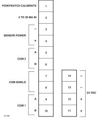
Figure 3-49—Wiring Configuration for DCU
