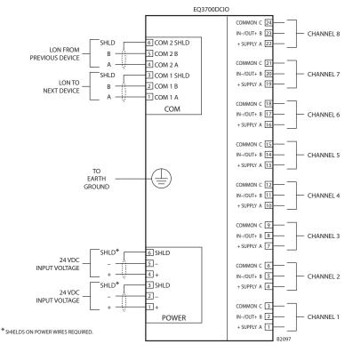
Figure 3-35—DCIO Module Wiring Terminal Configuration
