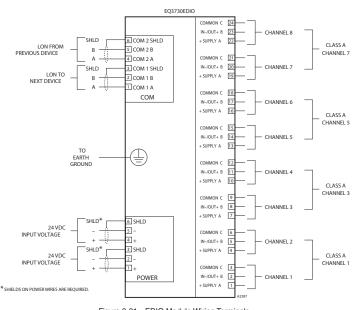
Figure 3-21—EDIO Module Wiring Terminals
