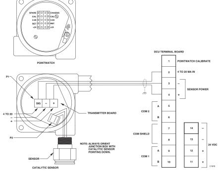
Figure 3-54—Sensor Separation Kits
