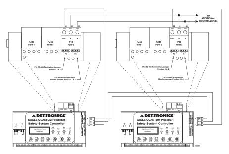
Figure 3-9B—Controller to Controller Communication with Class A Signaling Line Circuit Classification per NFPA 72, for Controllers with Ethernet Interface Board
