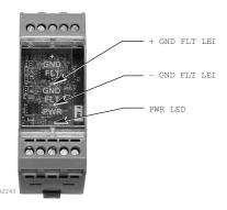
Figure 4-11—Ground Fault Monitor Status Indicator Location
