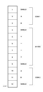
Figure 3-3—Network Extender Wiring Terminal Identification
