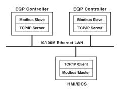
Figure 2-7—Ethernet TCP/IP Server/Client Relationship & Modbus RTU Master/Slave Relationship
