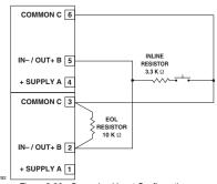
Figure 3-26—Supervised Input Configuration for Opens and Shorts – Class A
