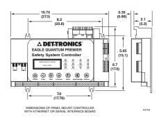
Figure 6-1—Dimensions of EQP Controller in Inches (Centimeters)
