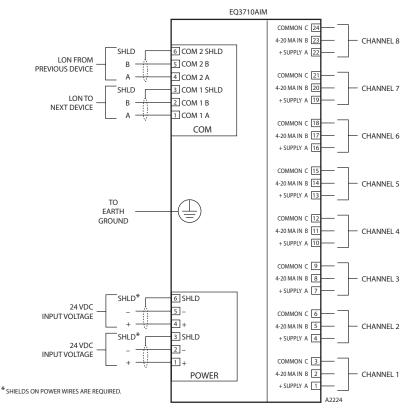
Figure 3-43—Analog Input Module Wiring Terminal Configuration
