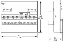
Figure 6-3—Dimensions of the EDIO / DCIO / Relay Module / AIM in Inches (Centimeters)
