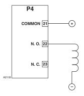
Figure 3-5—Unsupervised Relay Output
