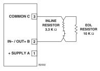
Figure 3-38—Supervised Input Configuration (Opens and Shorts)
