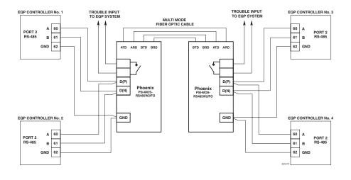
Figure 3-12—Multi-Mode Controller to Controller NFPA 72 Approved Fiber Optic Link, Class X
