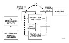
Figure 2-6— Block Diagram of EQP System with Redundant Controllers
