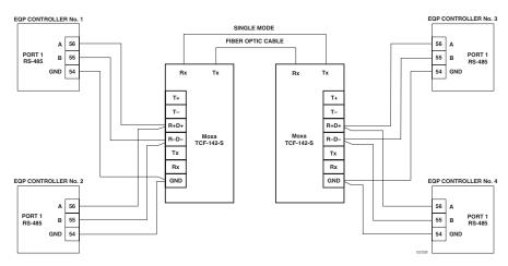
Figure 3-10—Controller to Controller NFPA 72 Approved Fiber Optic Link, Class B
