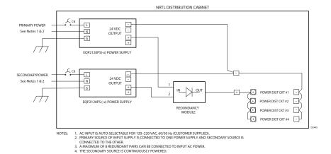
Figure 3-19A—Wiring Connections for a 20amp DC (Maximum) Power Supply with Primary and Secondary AC Sources
