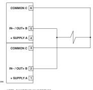
NOTE: SHUNT/FLYBACK DIODES DO NOT NEED TO BE INSTALLED ON THE FIELD DEVICE. CIRCUIT PROTECTION IS PROVIDED WITHIN THE EDIO MODULE.
