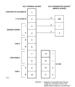
Figure 3-52—DCU Transmitter Board Connected to Terminal Wiring Board
