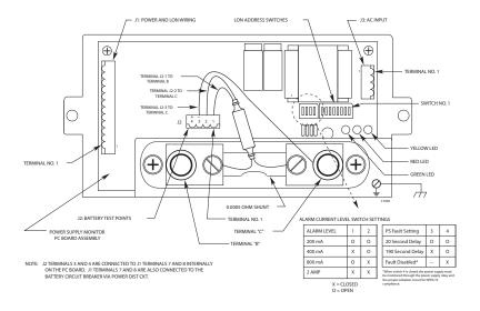
Figure 3-14—Power Supply Monitor Terminal and Switch Location
