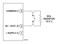
Figure 3-37—Supervised Input Configuration
