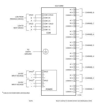
Figure 3-42— Relay Module Wiring Terminal Configuration
