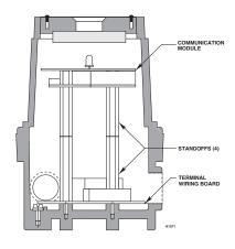
Figure 3-48—Printed Circuit Boards in Universal DCU
