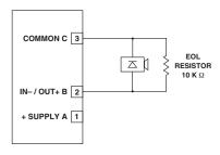
Figure 3-39—Supervised Output Configuration (Notification)
