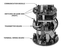
CORRECT ORIENTATION OF TRANSMITTER BOARD
