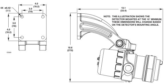
Figure 2—Q9033 Mounting Arm Dimensions in Inches (cm)
