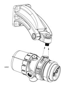
Figure 6– Connecting a Detector with Collar Attachment to Mounting Arm
