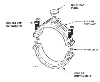
Figure 4–Collar Attachment Assembly
