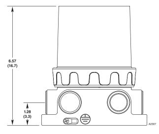
Figure 4—Termination Box Dimensions in Inches (cm)
