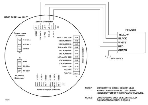
Figure 12—PIRDUCT Wired Directly to UD10
