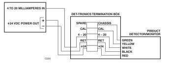
Figure 9—Typical Wiring, PIRDUCT with PIRTB Termination Box
