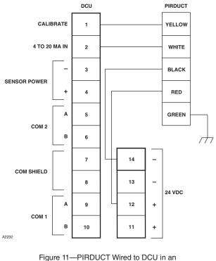
Figure 11—PIRDUCT Wired to DCU in an Eagle Quantum Premier System
