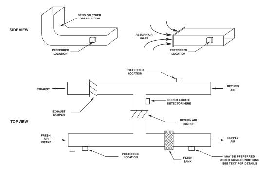
Figure 6—Detector Placement
