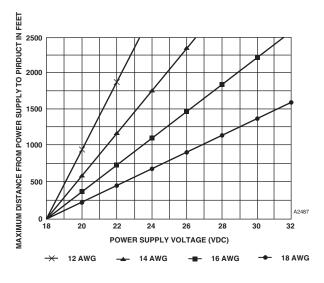
Figure 2—PIRDUCT Wiring Requirements
