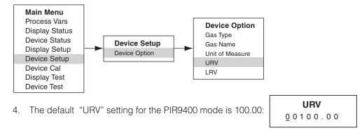
To change the setting, highlight a digit (indicated by the underline) by using the CANCEL/ESCAPE (move left) and ENTER/ SELECT (move right) switches. Each individual digit is changed by using the PREVIOUS (higher) and NEXT (lower) switches. Once the "URV" has been set to 15.00, use the ENTER/SELECT switch to save the new value.
