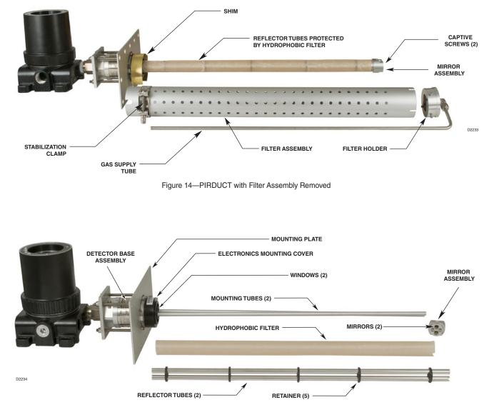
Figure 15—PIRDUCT Disassembled for Cleaning
