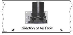
Figure 7—Orientation of PIRDUCT Mounting Plate Relative to Direction of Airflow through Duct
