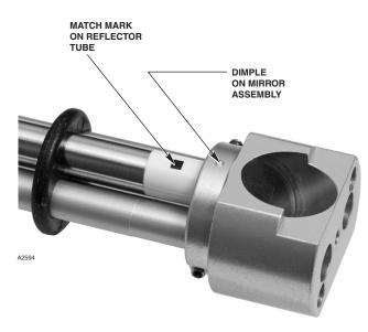
Figure 16—Match Mark on Reflector Tube Lines Up with Dimple on Mirror Assembly
