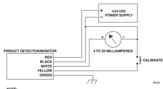
NOTE: CALIBRATION PUSHBUTTON, CURRENT METER AND POWER SUPPLY ARE NOT SUPPLIED.
