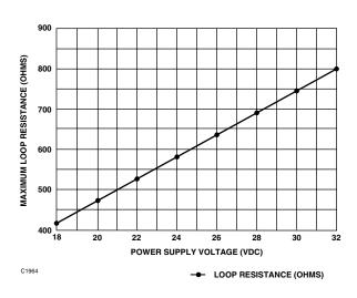
Figure 1-4 to 20 mA Current Loop Resistance
