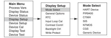
2. From the "Mode Select" menu, select PIR9400 as the operating mode to be used for the PIRDUCT connection to UD10-DCU. A "Successful" message will briefly appear on the display, confirming the change.
