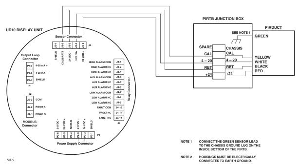
Figure 13— PIRDUCT Wired to UD10 through PIRTB Termination Box
