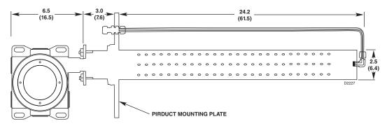
Figure 3—Dimensions of PIRDUCT in Inches (cm)
