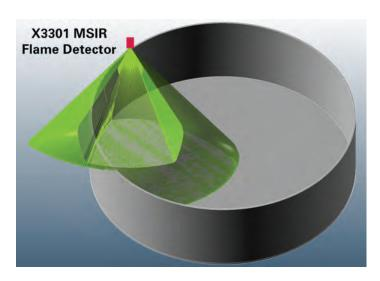
The detection range of the Det-Tronics X3301 Multispectrum Infrared Flame Detector (FM approved to detect a 1 ft<sup>2</sup> heptane fire at 265 feet (0.09 m<sup>2</sup> fire at 80.7 meters)) allows one detector to cover a large portion of the floating roof seal along with the surface of the floating roof and, in some cases, the area outside of the tank wall.
